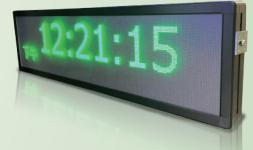
MEGA-3000 is a network-connected LED message display sign for indoor installation.
